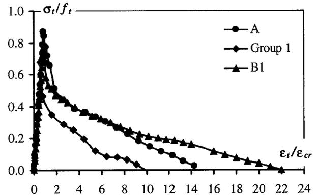
**Fig. 2.** Tension stiffening relationships for steel reinforced beams
