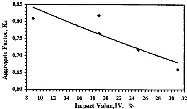
**Fig. 1.** Correlation between aggregate factor corresponding to the Bolomey formula and aggregate impact value
