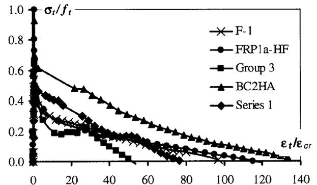
**Fig. 1.** Tension stiffening relationships for FRP reinforced beams
