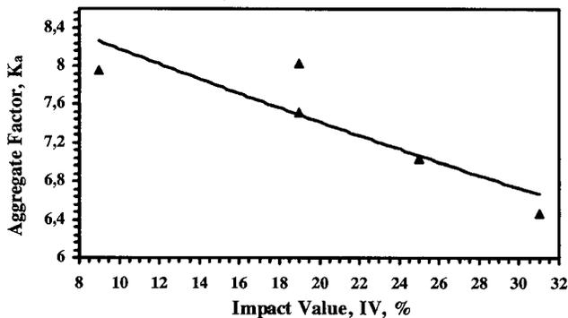
**Fig. 2.** Correlation between aggregate factor corresponding to the Feret formula aggregate impact value
