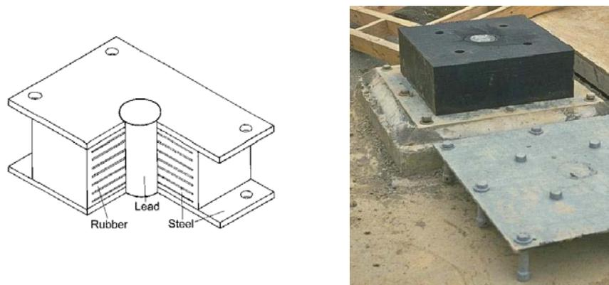
Figure 1, Lead Core Steel Laminated Elastomeric Isolation Bearing
