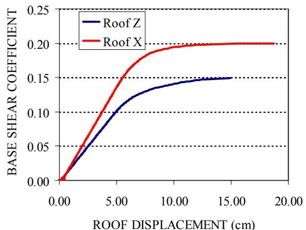
Figure 5, Pushover Curve for Non-Isolated Building
