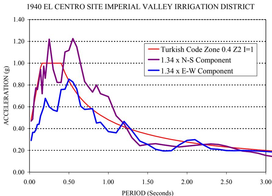
Figure 7, 5% Damped Spectrum of Time History Used for Analysis
