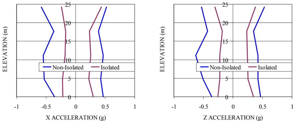
Figure 10 : Maximum Acceleration Profiles
