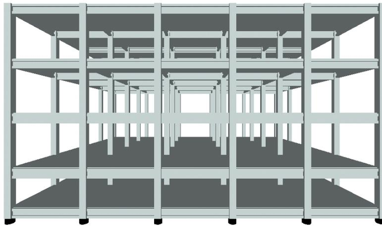
Figure 6, Analysis Model of Isolated Building
