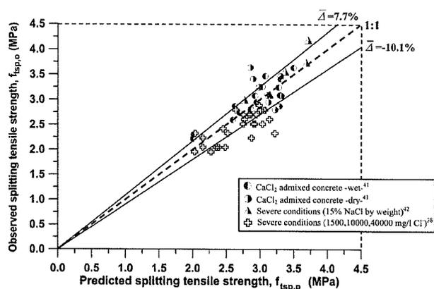
Fig. C—Comparison between experimental data gathered from various sources and these predicted values from modified Eq. (7)<sup>36</sup> (deviation  $\Delta = (f_{sp,o} - f_{sp,p})/f_{sp,o} \times 100$ , %).
