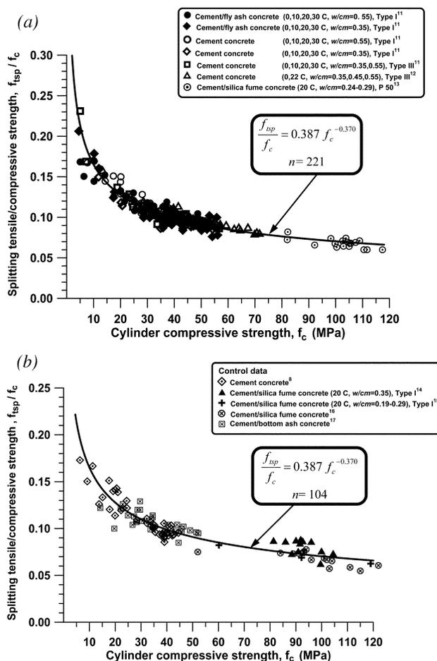
**Fig. 1—Ratio of splitting tensile to compressive strength versus cylinder compressive strength: (a) group I used to obtain A and B; and (b) compared with verification data II.**
