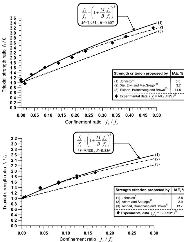
Fig. 3—Experimental data of concretes under triaxial compression compared with strength criteria proposed by various researchers.
