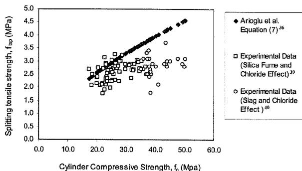
Fig. A—Relation between tensile and compressive strength of concrete exposed to chloride.
