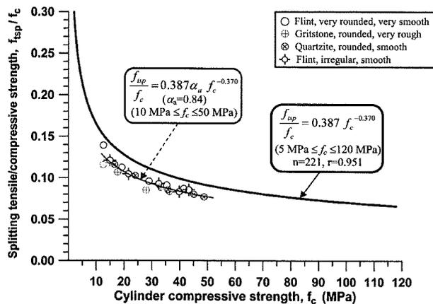
Fig. D—Modified relationships between ratio of splitting tensile ( $\phi 150 \times 300$  mm) to compressive strength ( $\phi 150 \times 300$  mm) and cylinder compressive strength for concretes made with uncrushed gravel aggregates ( $\alpha_c$  = calibration factor taking aggregate shape and texture into consideration.)
