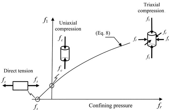
Fig. 2—Johnston's strength criterion to estimate ultimate axial compressive strength for intact rock under triaxial compression.
