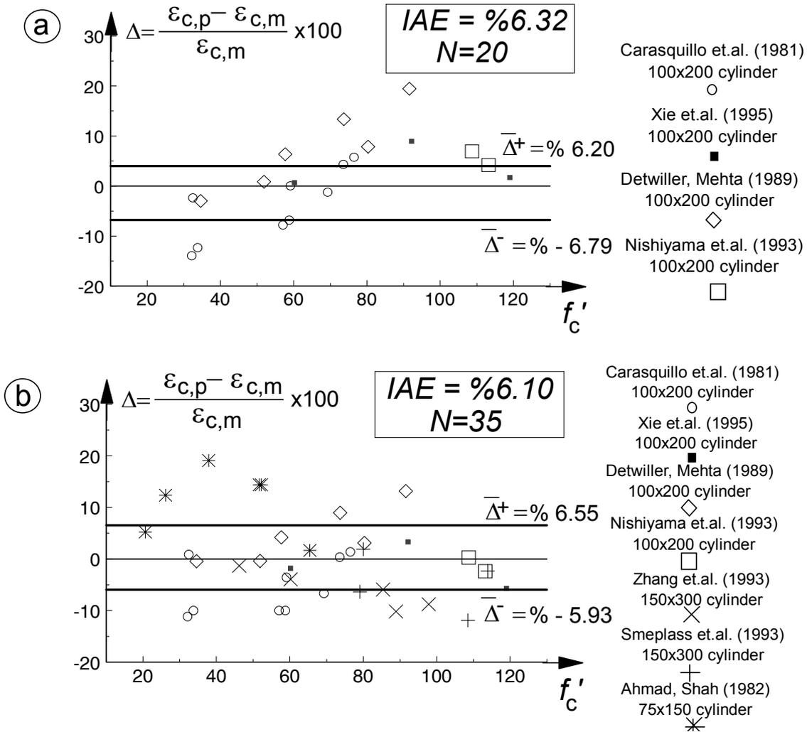
Fig.C - Error Analysis for Attard-Setunge's Equation (a) and for Arıoğlu's Equation (b)
