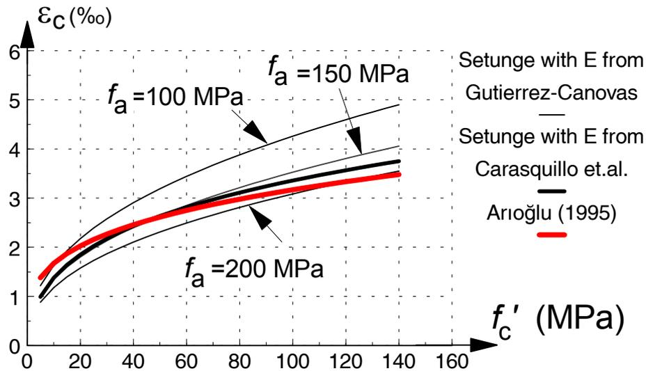
Fig.D - Strain at Peak Stress with Different " $E_c$ " Equations
