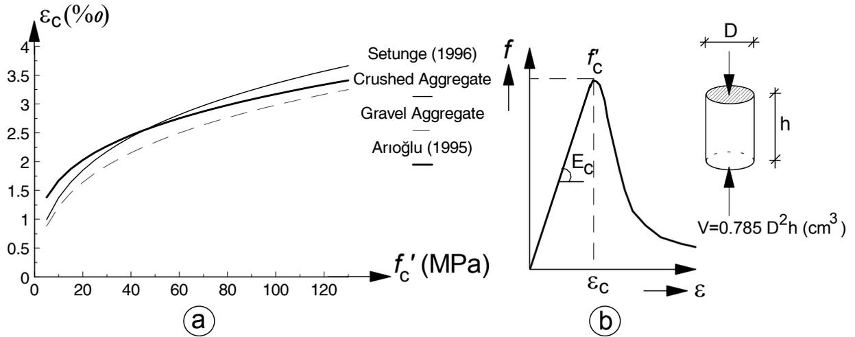
Fig. B- Comparison of Setunge's Equations ( $E_c$  from Carasquillo et.al.) with Equation Proposed by Arıoğlu<sup>33</sup>
