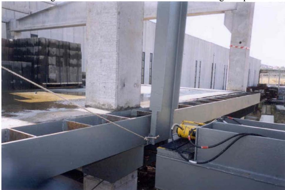
Figure-5: Full Scale Test Structure and Loading Setup
