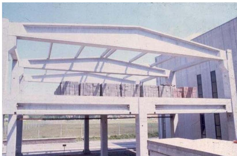
Figure-2: Full Scale Test Structure and Loading Setup
