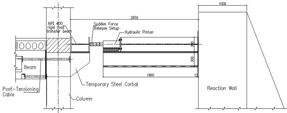
Figure-9: Lateral Load Application Detail
