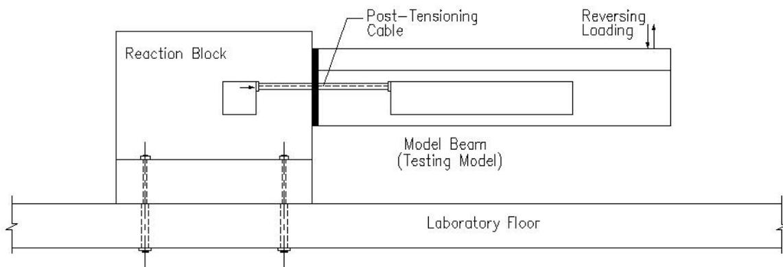
Figure-1: Test Unit on 1/ 2.5 Scale
