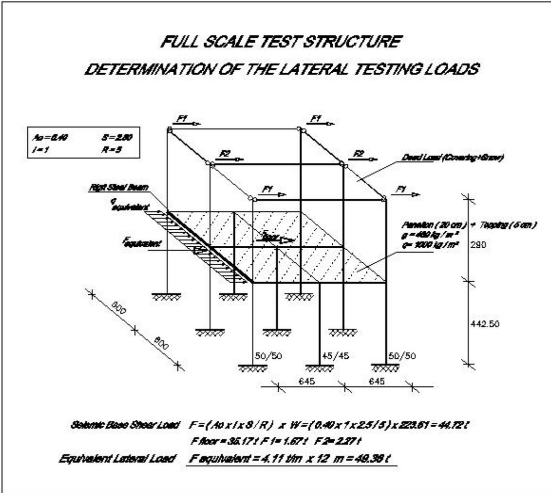
Figure-10: Static Lateral Loads Applied for the Tests
