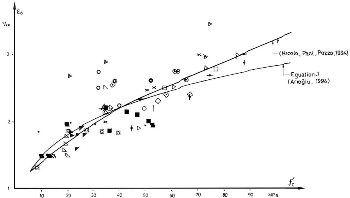
Fig.  $f'_c$  -  $\epsilon_0$  data of de Nicolo, Pani and Pozzo (see [1], Fig.4) shown with values calculated using Equation 1.
