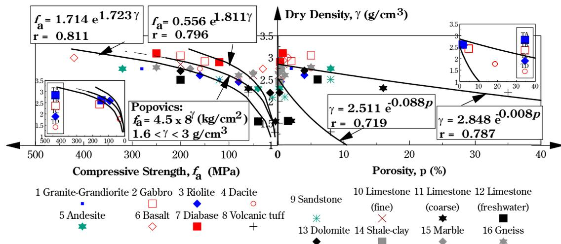
Fig. A—Relationships between the aggregate's physical and mechanical properties
