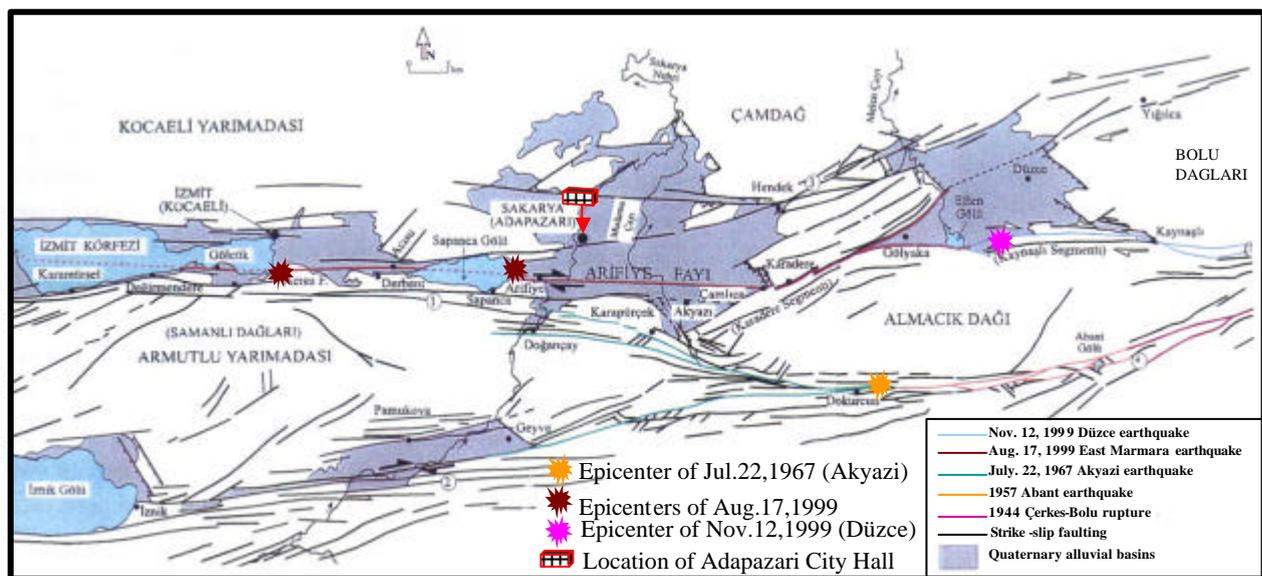
Fig. 1 The neotectonic map of Gerede-Izmit Bay region and earthquakes in the period of 1944-1999 (modifying [11] )
