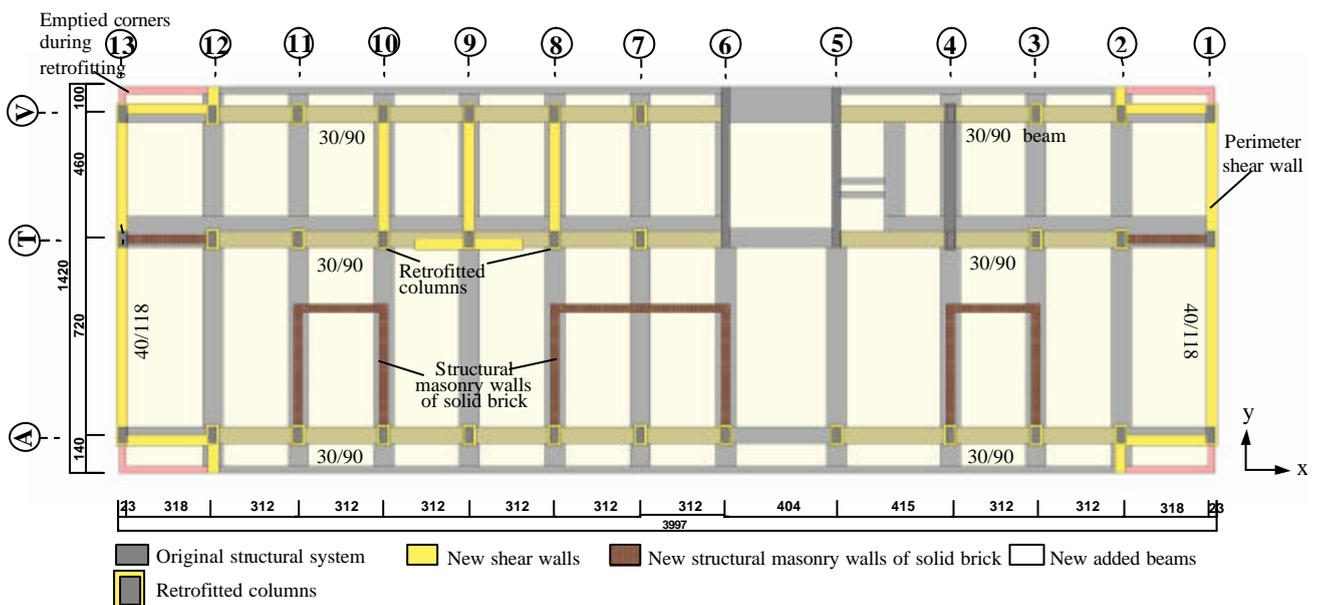
Fig.5 Main strengthening and repair works applied to Adapazari City Hall (the ground floor framing plan)
